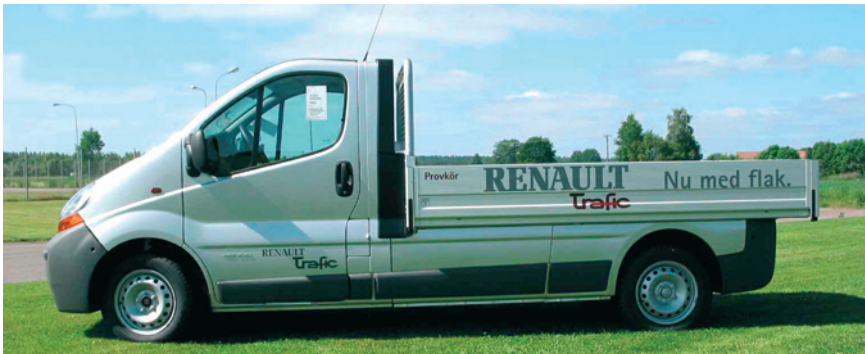
Fig. 5. The side panel below the loading area of the Renault Trafic consists of coextruded and thermoformed ABS/PMMA sheets
